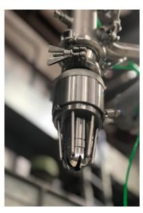
Single quick-release nozzles of various configurations are used to release ice cream in the form of roses. Group nozzles are used to produce one-color ice cream cakes with a different number of roses.
